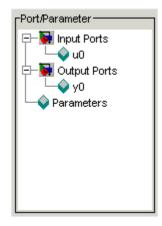
The pane contains a tree control whose top nodes correspond to the target S-function input ports, output ports, and parameters, respectively. Expanding the Input Ports, Output Ports, or Parameter node displays the input ports, output ports, or parameters, respectively, specified for the target S-function. Selecting any of the port or parameter nodes selects the corresponding entry on the corresponding port or parameter specification pane.
