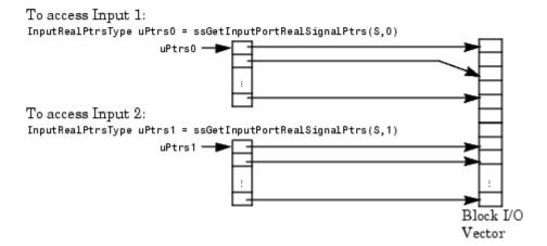
As shown in the previous figure, the input array pointers can point at noncontiguous places in memory.
